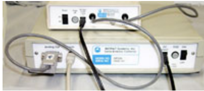
BSLSTM Trigger cable connection
