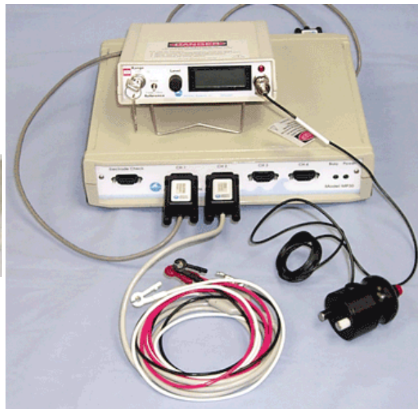
BSLSTM Reference cable, SS2L lead and HSTM01 stimulating probe connections
